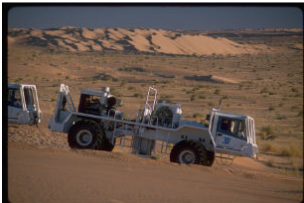
These truck mounted vibrators benefit from low ground pressure tires which can significantly increase recovery time from any impact.
